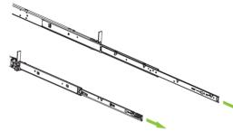
4 Align the rail standoffs on each side of the system and lower them into the slots on the rail. Put the system downward until all the rail standoffs are seated in the slots.
